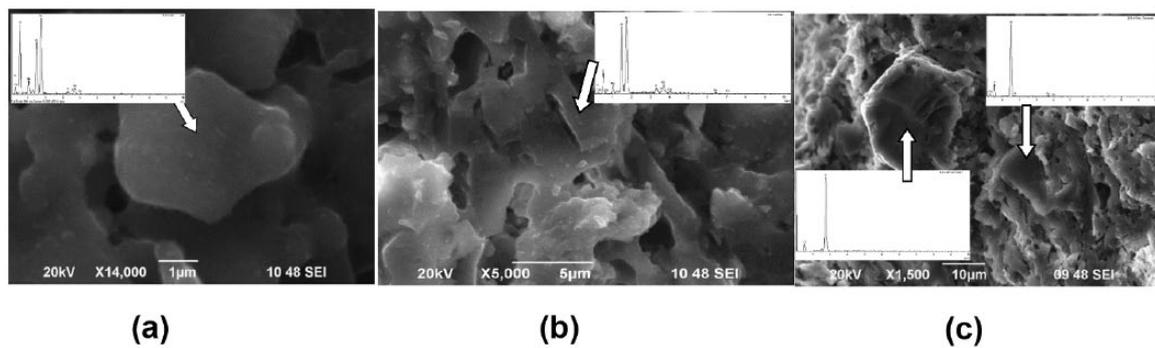
**Figure 6.** SEM images and EDS analysis of fractured surface of samples fired at 1000 °C: (a) C-b, (b) C-b-Na and (c) C-b-Al.
