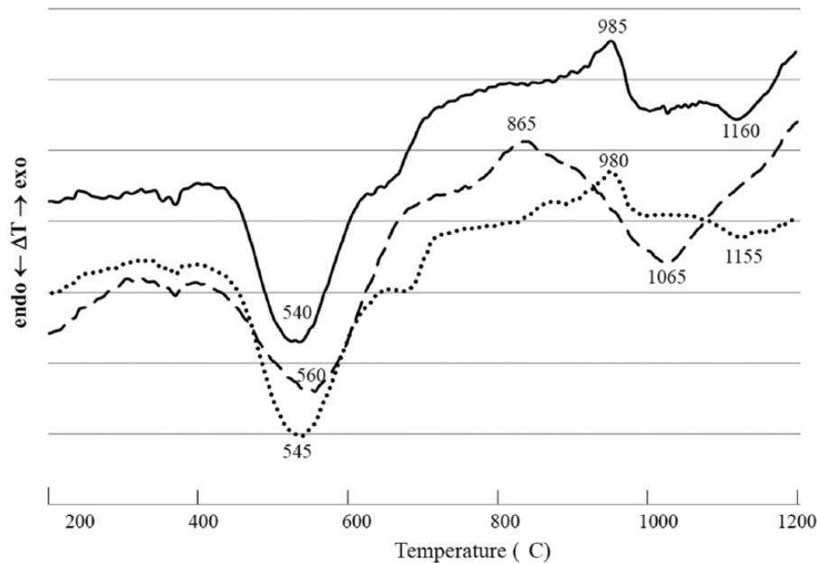
**Figure 4.** Non-isothermal DTA results of C-b (dot line), C-b-Al (solid line) and C-b-Na (dash line) ceramic batches.
