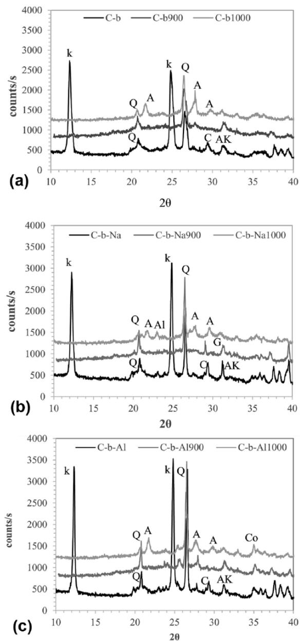
**Figure 5.** XRD spectra of (a) C–b, (b) C–b–Na and (c) C–b–Al ceramic batches at different temperatures. Q: quartz; K: kaolinite; A: anorthite; G: ghlenite; C: calcite; AK: Akermanite, Al: Albite, Co: Corundum.
