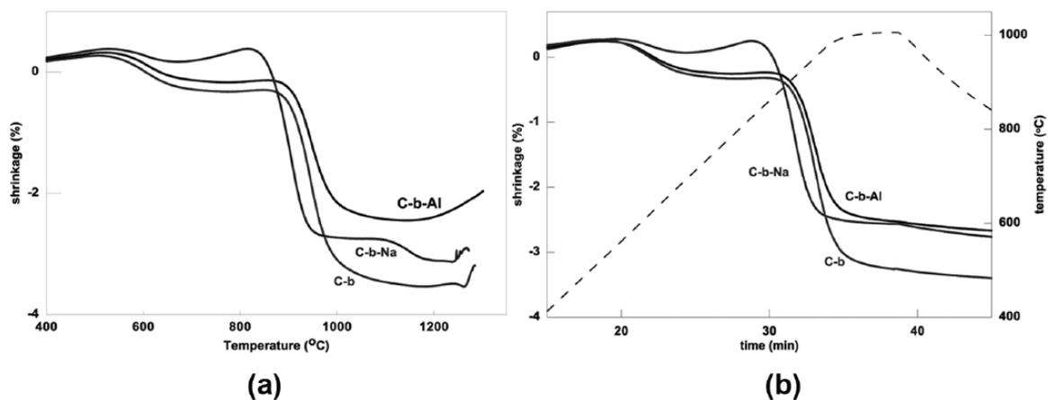
**Figure 3.** Dilatometer (DIL) curves of C–b, C–b–Al and C–b–Na compositions: (a) non-isothermal and (b) isothermal results after 5 min holding at 1000 °C.
