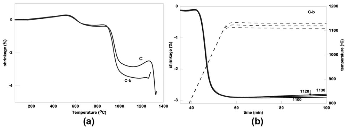
**Figure 2.** Dilatometer (DIL) curves of C and C–b compositions: (a) non-isothermal and (b) isothermal results at 1100 °C, 1120 °C and 1130 °C.
