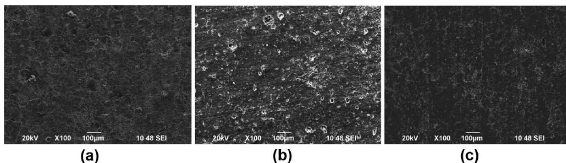
**Figure 7.** SEM images of samples surface fired at 1000 °C: (a) C-b, (b) C-b-Na and (c) C-b-Al.
