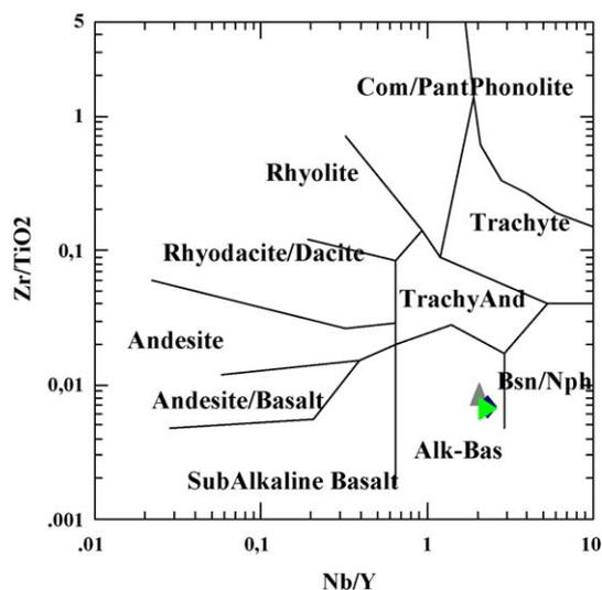
Fig. 1. Nb/Y–Zr/TiO<sub>2</sub> diagram highlighting the tuff composition.
