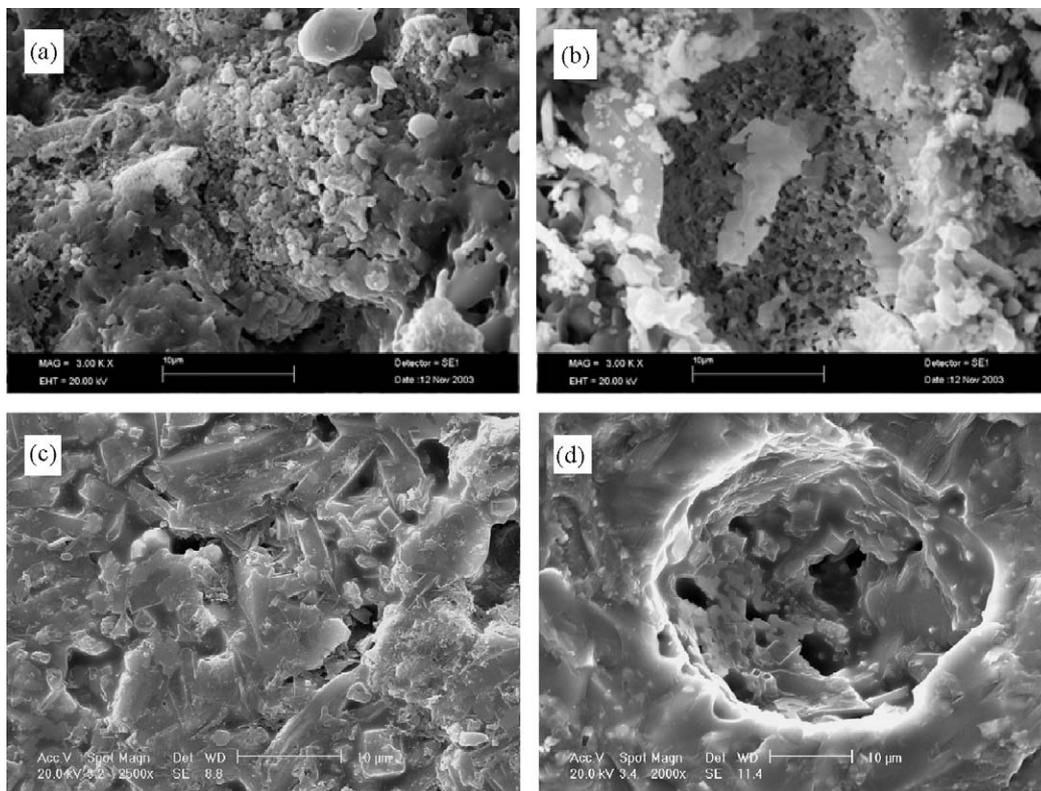
Fig. 9. SEM images of the BC surface (a), fracture (b), BT-gc surface (c) and fracture (d).
