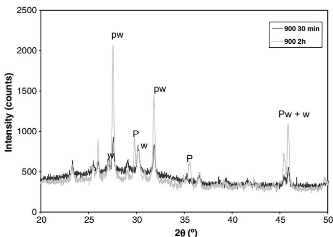
Fig. 5. XRD patterns of V1 glass-ceramics treated at 900 °C for 30 min (black line) and 2 h (gray line).
