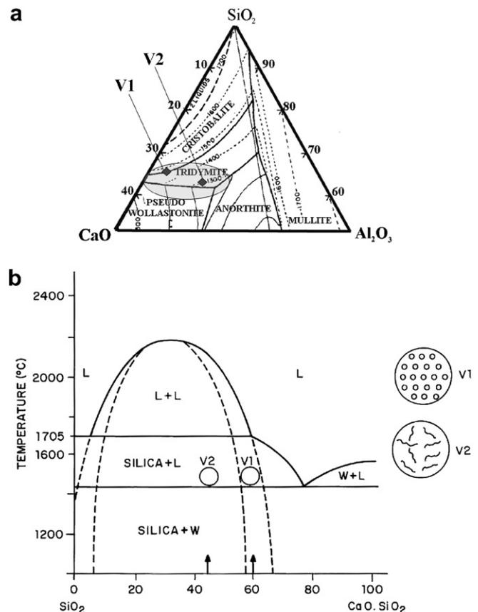
Fig. 6. (a) ternary diagram  $\text{SiO}_2$ – $\text{CaO}$ – $\text{Al}_2\text{O}_3$  and (b) binary immiscibility curve.
