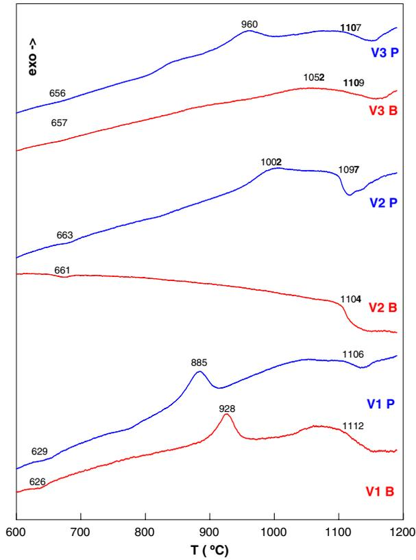
Fig. 3. DTA traces of powder and bulk samples at 10 °C/min.
