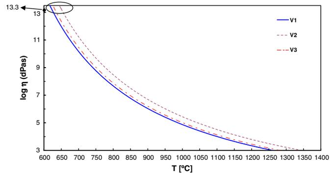
Fig. 2. Hypothetical viscosity–temperature curves of the studied compositions.
