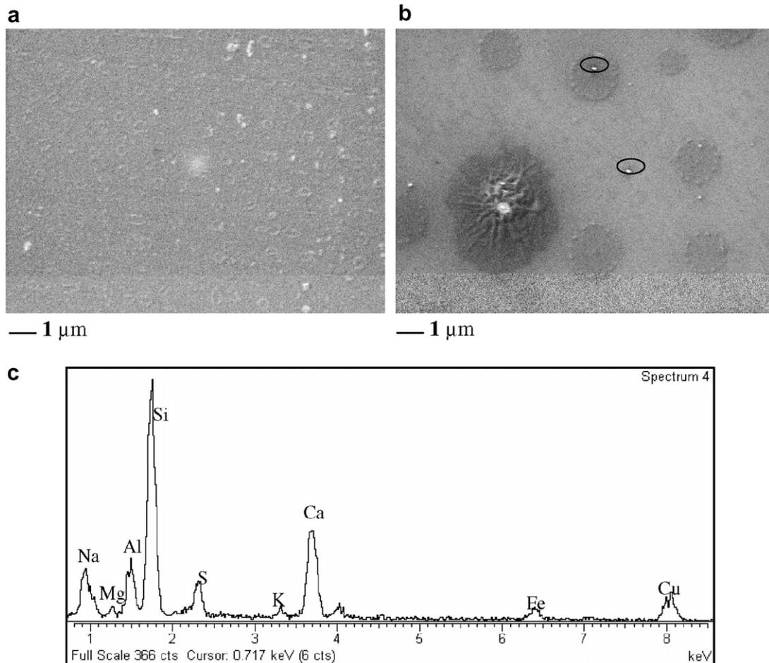
Fig. 1. SEM micrographs of V1 parent glass at 9000 $\times$  (a) and V2 parent glass at 5000 $\times$  (b). EDS spectrum of white dots (c).
