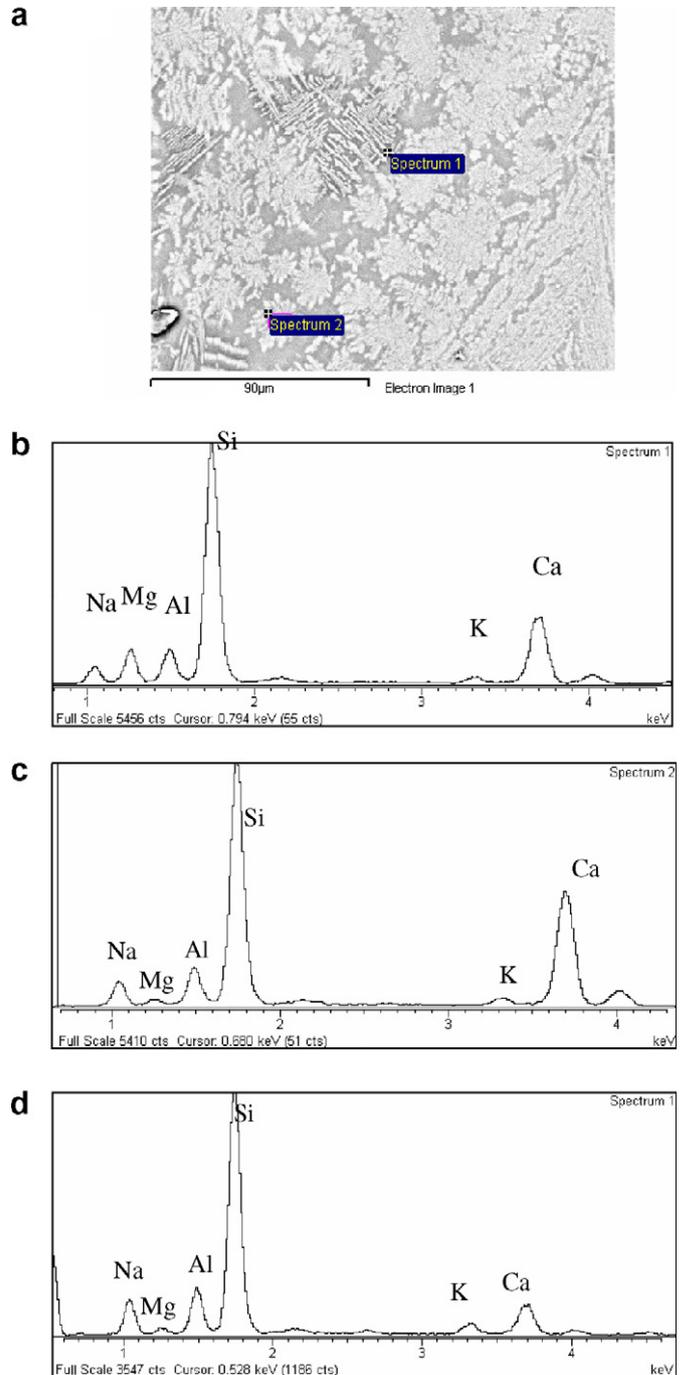
Fig. 4. (a) SEM micrograph of V1 glass-ceramic treated at 900°C for 2 h, (b) and (c) EDS spectra of different crystals, (d) EDS spectrum of the glass matrix.
