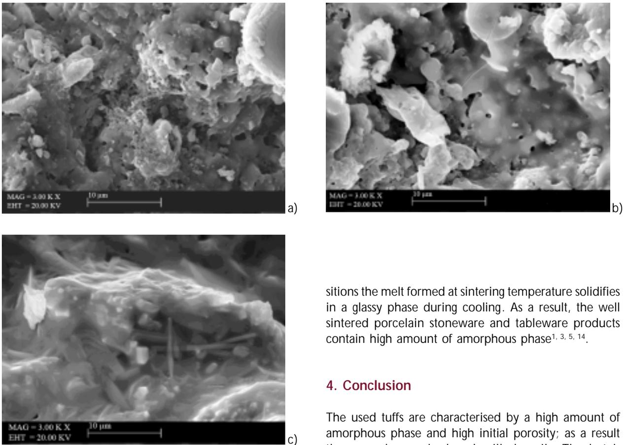
Figure 9. Fracture images of samples, fired at 900 °C (a), 1100 °C (b) and 1150 °C (c)
