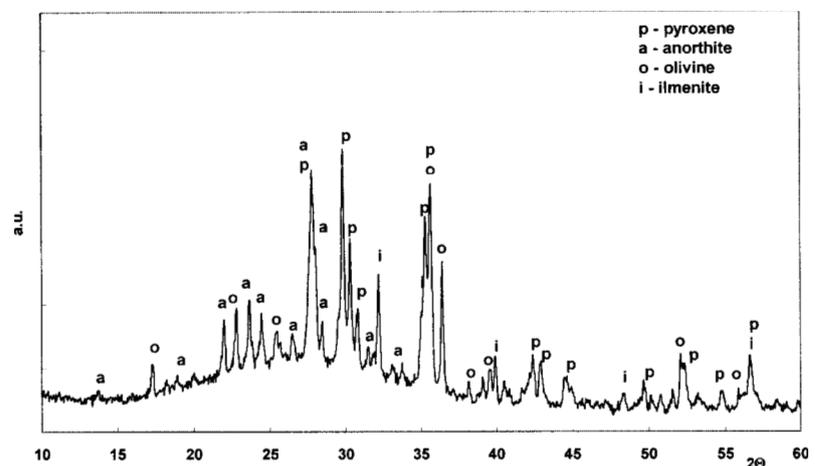
Figure 1. XRD spectra of the tuffs
