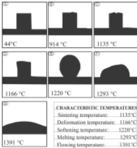
Figure 6. Hot-stage microscopy analysis of the ceramic sample
