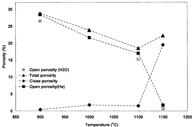
Figure 8. Total porosity ( $P_T$ ), closed porosity ( $P_C$ ) and open porosities for He ( $P_{He}$ ) and water ( $P_{H_2O}$ ) after 2 h holding at different sintering temperatures
