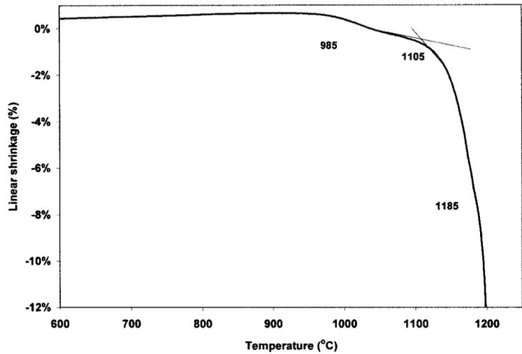
Figure 7. Dilatometry of the ceramic sample
