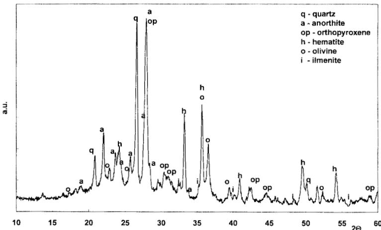
Figure 10. XRD analysis of the ceramic fired for 30 min at 1150 °C
