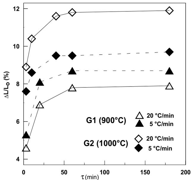
Fig. 6. Linear shrinkage as a function of the holding time at 900°C for G1 and 1000°C for G2.
