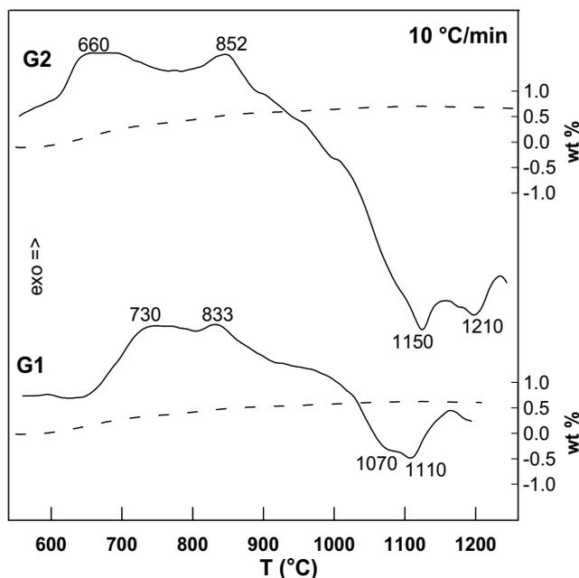
Fig. 1. DTA traces of the parent glass powders G1 and G2 in the range 550°–1250°C.
