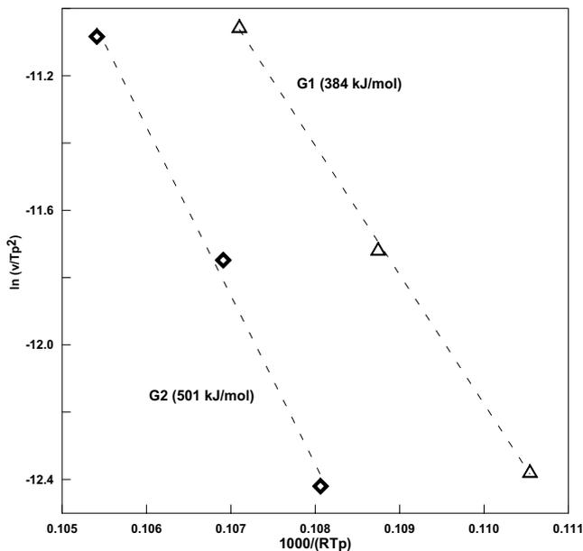
Fig. 4. Kissinger plots and the activation energy of crystallization,  $E_C$ , of G1 and G2.
