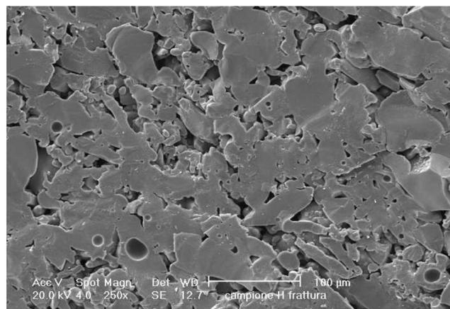
Fig. 9. SEM image of fractured G2 glass-ceramic, heated at 5°C/min and sintered 1 h at 1050°C. (SEM images at 950° and 1000°C are available in the Data Depository.)
