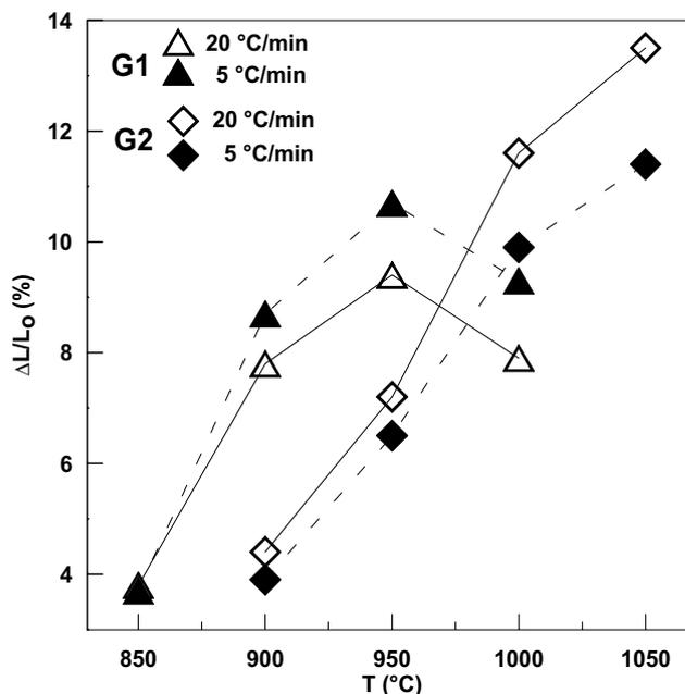
Fig. 5. Linear shrinkage as a function of a 1-h step of the holding temperature.
