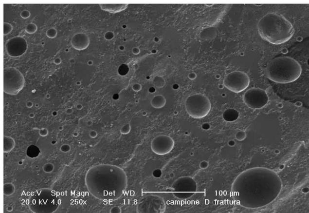
Fig. 8. SEM image of fractured G1 glass-ceramic, heated at 5°C/min and sintered 1 h at 1000°C. (SEM images at 900° and 950°C are available in the Data Depository.)
