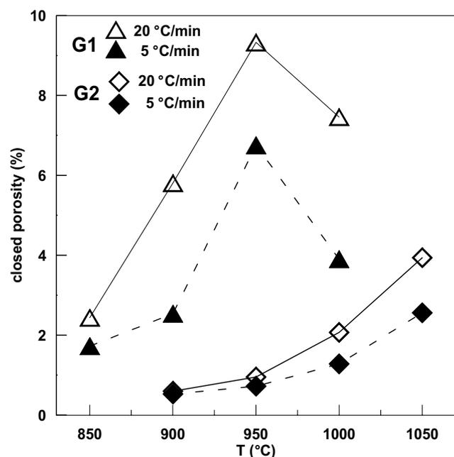
Fig. 7. Percentage of closed porosity after a 1-h step as a function of the holding temperature.
